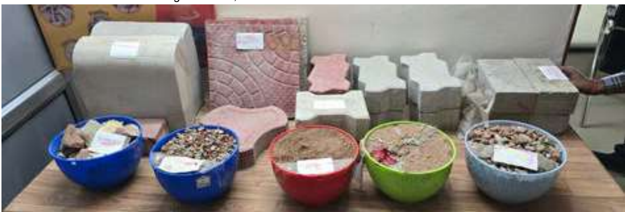
Picture 47: Paver tiles and bricks created from C&D waste, Source: NIUA
